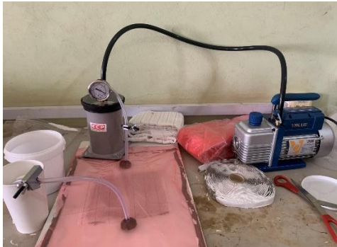
Figure 1a. VARTM process
