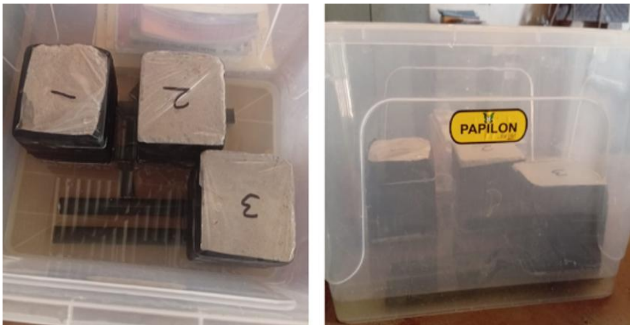
Figure 3 (a) and (b) Test set-up for capillary sorption test
