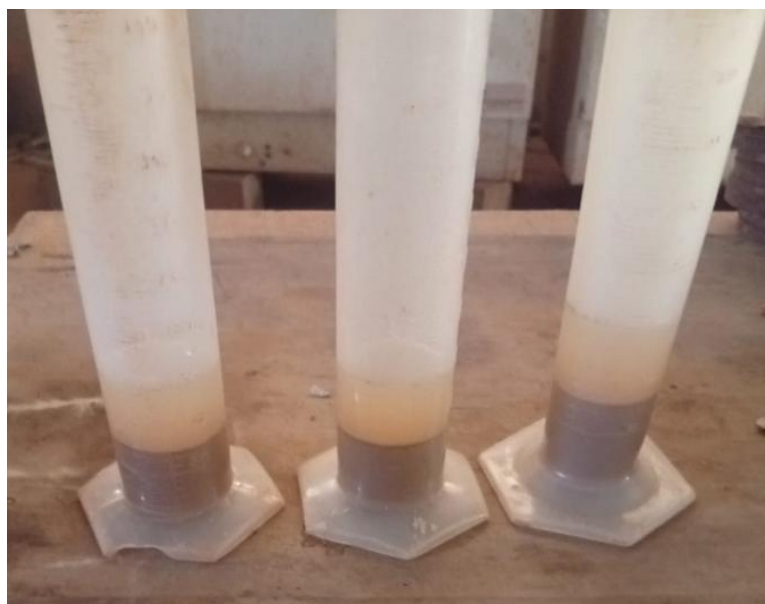
Figure 2: Set up for sedimentation tests for fine and sharp sand
