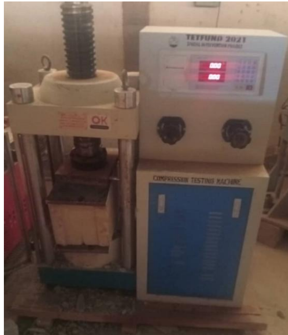
Figure 4: Set-up for compressive strength test of hollow concrete blocks
