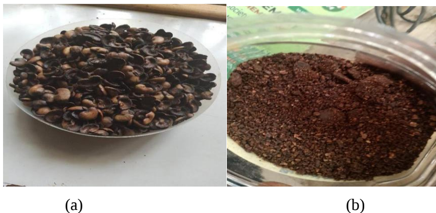
Plate 1: Samples: (a) Cleaned and sun dried cashew nutshells; (b) Milled cashew nutshells
